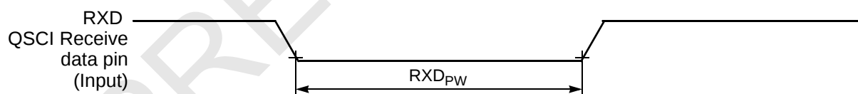
Figure 10-12 RXD Pulse Width
