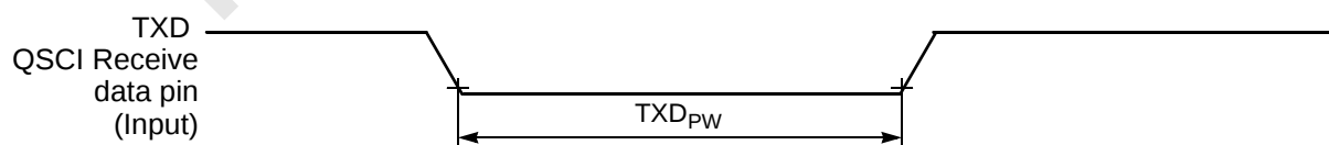
Figure 10-13 TXD Pulse Width
